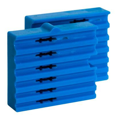
This is the replacement blade set for the MS-6 Fiber Optic Mid Span Slitting Tool and comes with (2) blade cartridges. This replacement blade set is for cable diameters from 1.2 mm to 3.3 mm. The blades are made for long term use and last for up to 5,000 slits/cuts.
