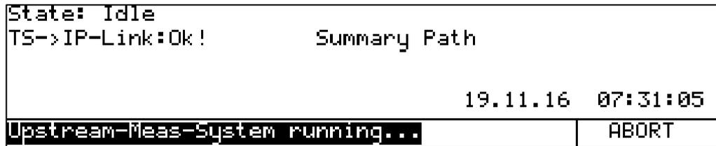
Figure 6-15 Start display of the LC display in the summary mode of the SW 024 (TS output via IP)
