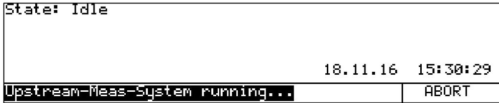
Figure 6-4 Start display of the LC display after starting the UMS (TS output via ASI)
