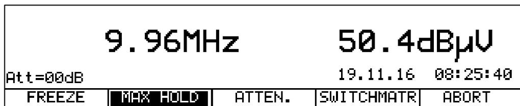
Figure 7-5 Activation of the MAX-HOLD function in the real-time analyzer
