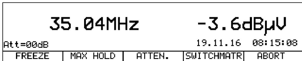
Figure 7-2 LC display content after call-up of the return path spectrum analyzer
