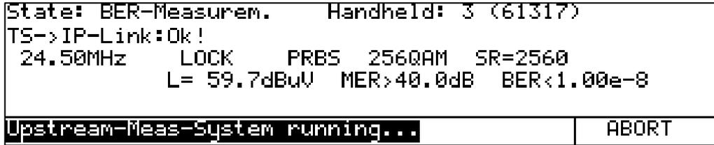
Figure 6-11 LC display during MER/BER measurement by a field instrument
