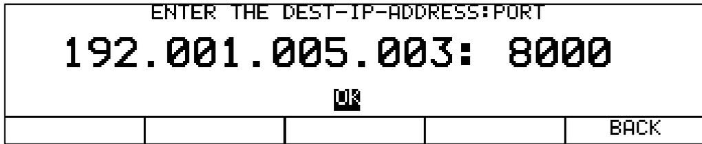
Figure 8-1 Input of the destination IP address and port for the TS streaming interface
