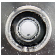
Top of the contaminated connecting bar
