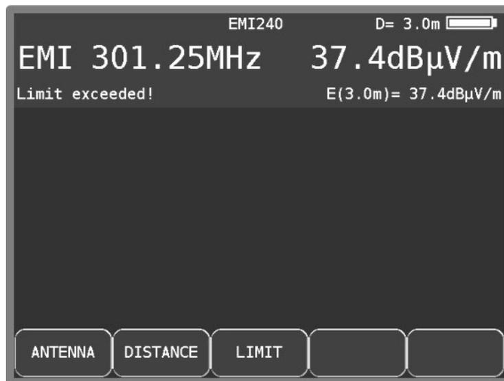
Figure 10-3 EMI measure field strength
