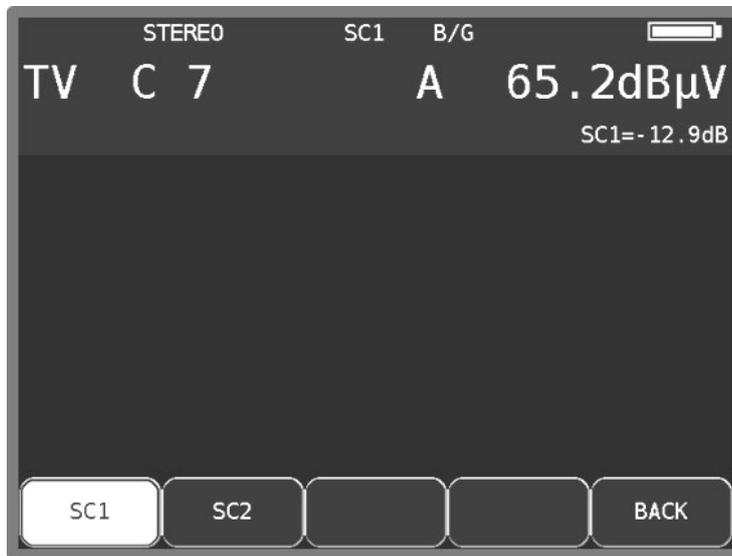
Figure 7-2 Display sound carrier
