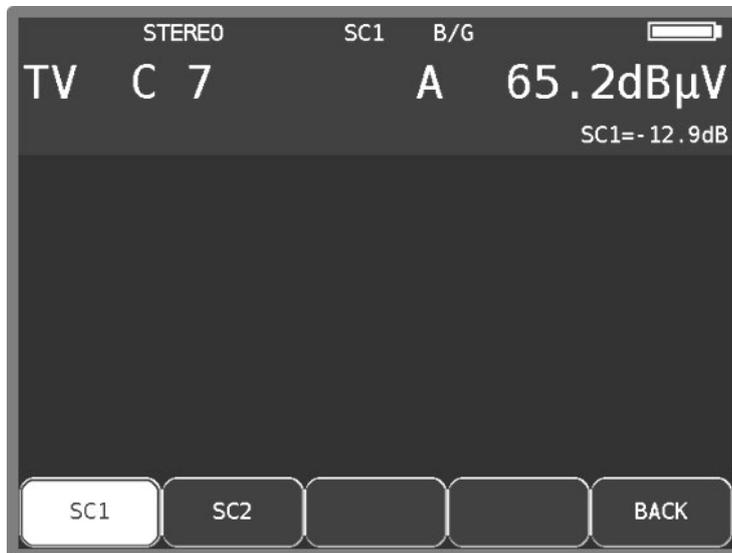
Figure 7-2 Display sound carrier
