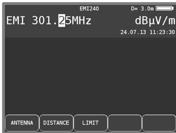
Figure 10-1 Electromagnetic interference measurement main screen
