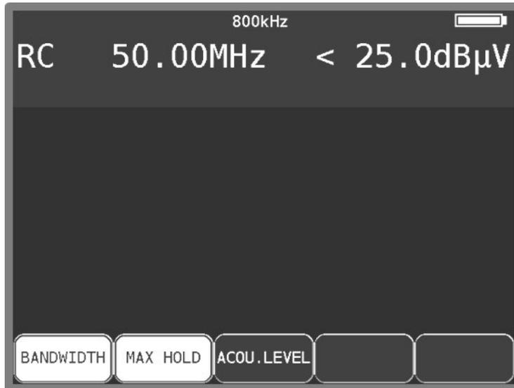
Figure 9-2 RC Max Hold function
