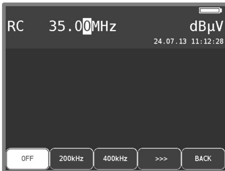
Figure 9-3 RC Setting channel bandwidth
