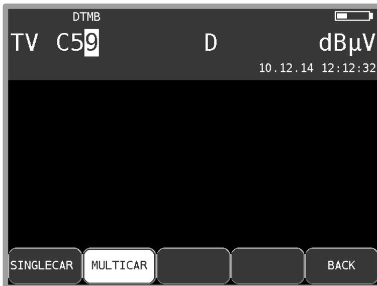
Figure 7-26 DTMB selecting carrier mode
