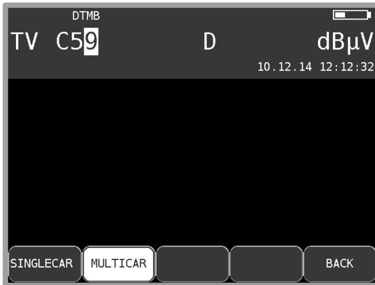
Figure 7-26 DTMB selecting carrier mode
