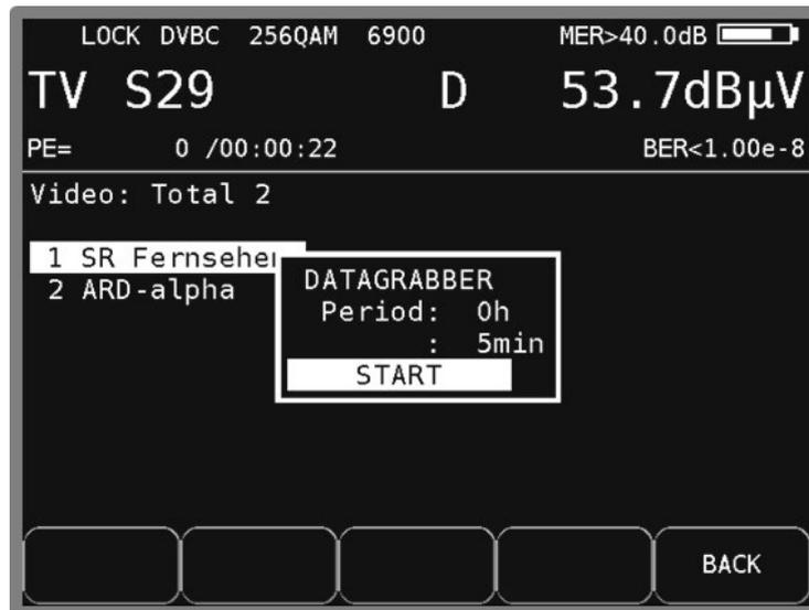
Figure 20-1 DataGrabber configuration of measurement time
