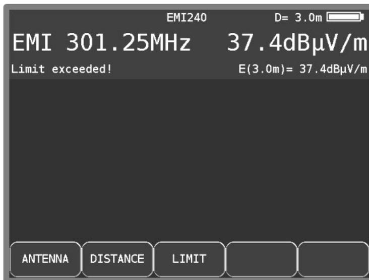
Figure 10-3 EMI measure field strength
